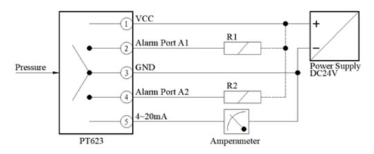
The load R1 (or R2) should be connected between the alarm port A1 (or A2) and VCC port. The action pressure of each alarm port can be set separately.
